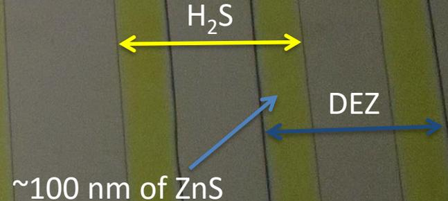
Picture showing ZnS "stripes", deposited to check performance of the coating system
