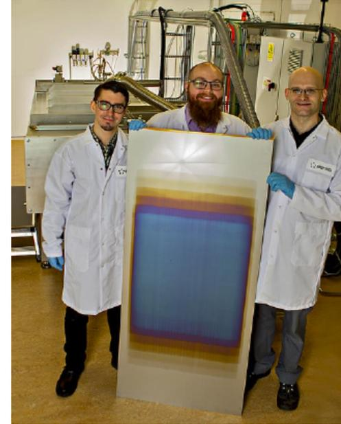
70 nm on ZnO on stainless steel showing effective coating area
