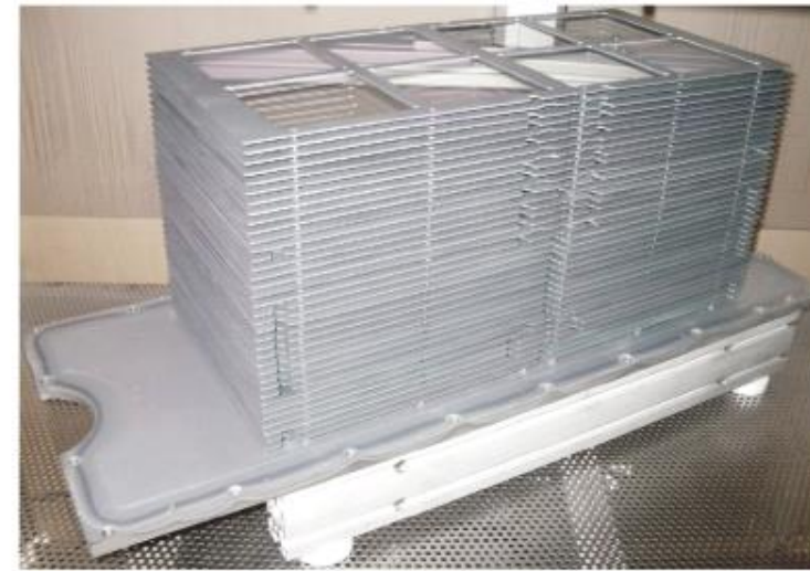
Fig. 4. Example of the \text{TiO}_2 batch for uniform ( \pm 2\% ) coatings, 36 shelves 240 \times 500 (mm), double-sided coatings ( 8 \text{ m}^2 of a film). 1
