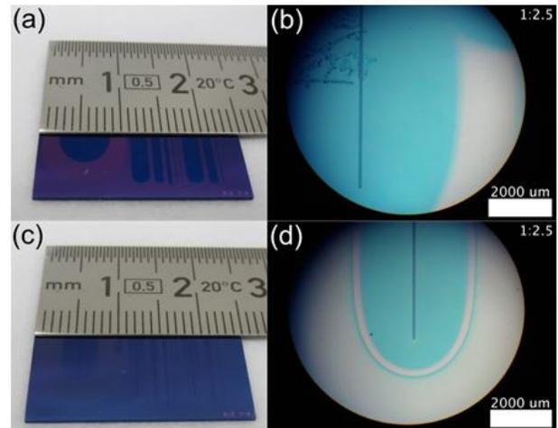
Figure 2: ALD  $\text{Al}_2\text{O}_3$  (a-b) and  $\text{TiO}_2$  (c-d) growth into LHAR structures with a maximum AR of 1:5000.
