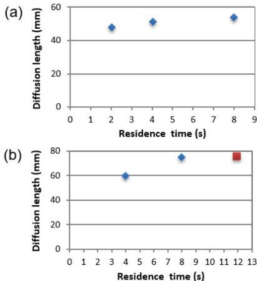
Figure 1: Influence of residence time on the diffusion length of stop-flow ALD grown  $\text{Al}_2\text{O}_3$  (a) and  $\text{TiO}_2$  (b) into a high AR lateral hole.
